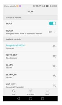
After connection succeeded, it will head to the login page automatically. Select the SSID of your Wi-Fi and enter the passwd, click OK.
